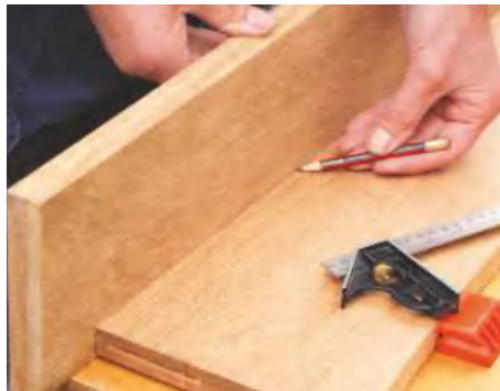
STEP 8. Saw the shelf to length and plane the end-grain. Mark out biscuit positions on the shelf and back panel
